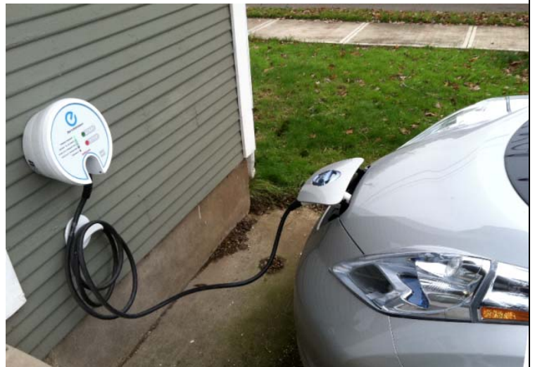
Electric cars vary on their recharging times—from a “quick charge” 30 minutes to a “home plug” 20 hours—depending on the station type. Sparky can go from empty to full in about six hours with this model.
